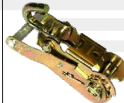
Part # 38-20SJ1 2" Wide Handle with Swivel J Hook WLL: 3670 lbs
