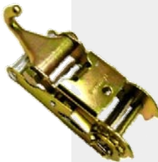
Part # 38-17 2" Ratchet with Forged Finger Hook WLL: 2,000 lbs
